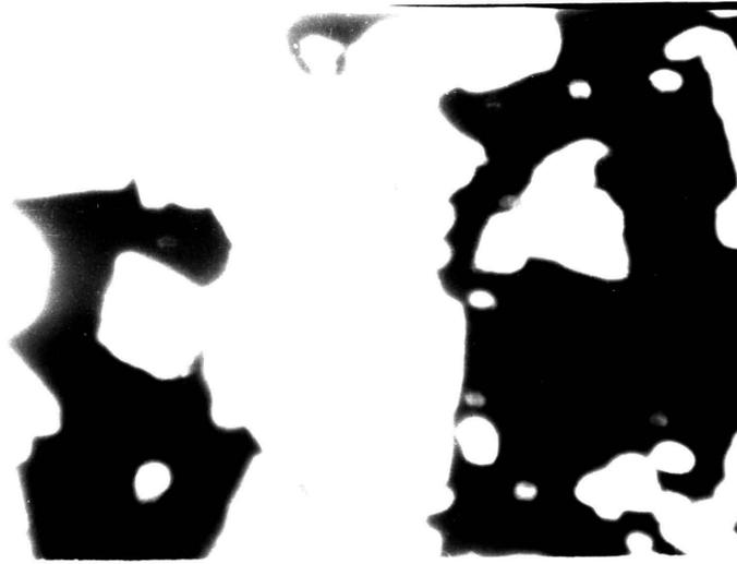
Figure 53- photomicrograph of a thin section showing amphiboles (white) which is surrounding and replacing magnetite (black). Mastuerzo zone, Vein IA, 944 level, specimen A-11. Plane polarized light. 32 X.
