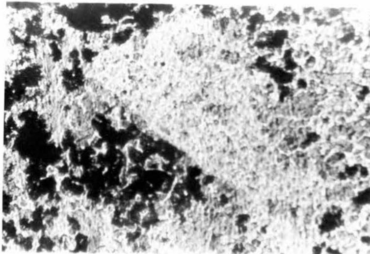
Figure 32. - Photomicrograph of a polished section showing magnetite with colloform and microporous texture. Mastuerzo zone, Vein 1A, 744 level, specimen A-56. Plane polarized light, 100X.
