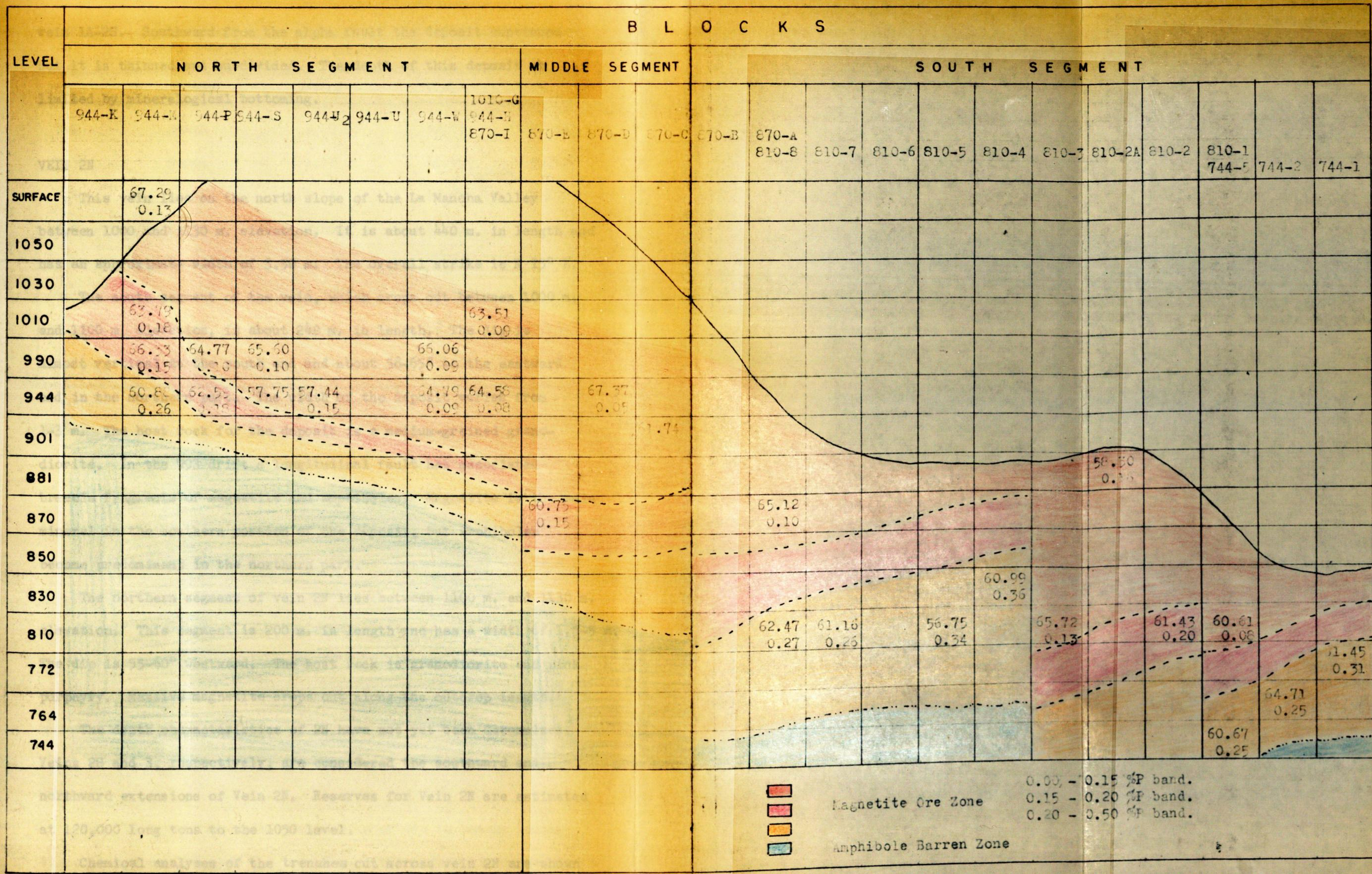
FIGURE 60.- Schematic longitudinal profile of the phosphorus banding in the magnetite Ore Zone of vein 1A-2S, Pastuerzo zone, Acari Iron Mining District.
