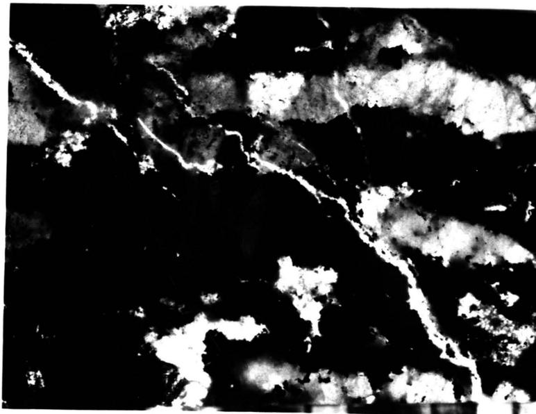
figure 48- photomicrograph of a thin section showing cavities between the scalloped layers of magnetite (black) filled by quartz (white). Mastuerzo zone, Vein 1A, 870 level, specimen A-20.
