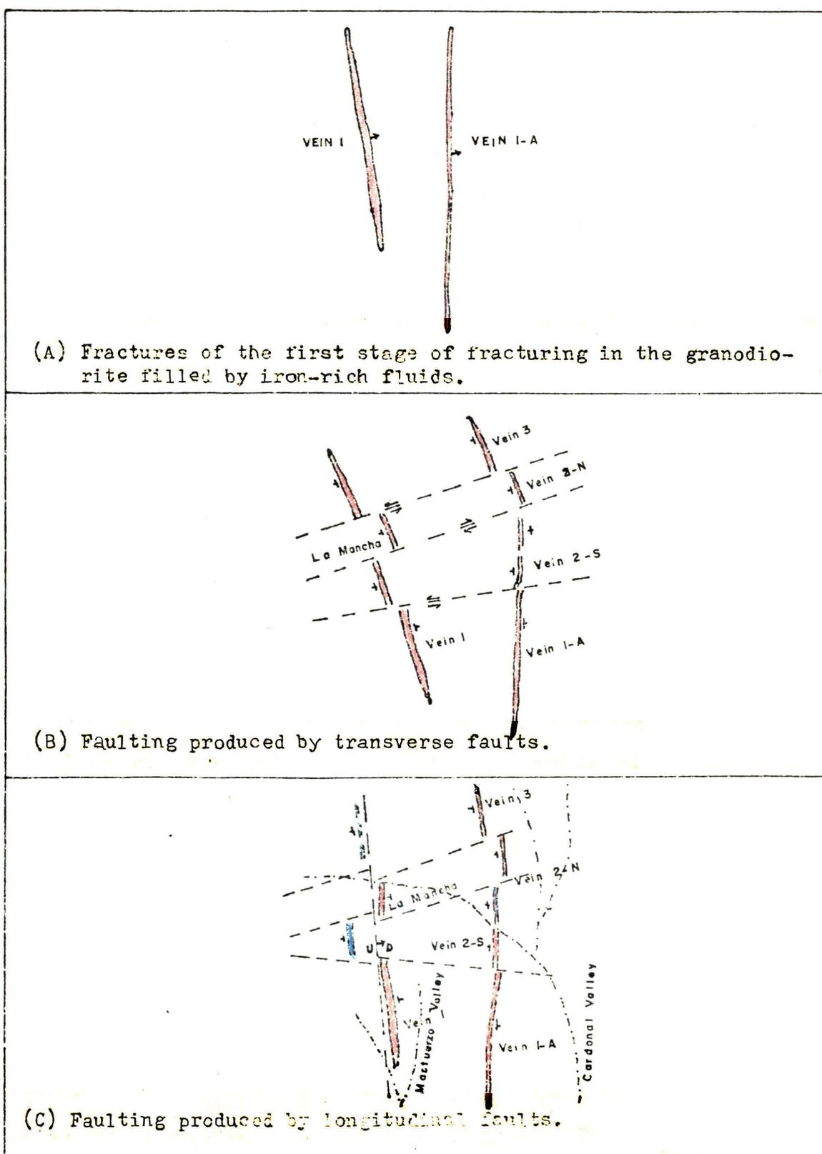
FIGURE 1C.— Diagram showing the different stages of faulting of the veins 1 and 1-A, Mastuerzo zone, Acari Iron Mining District.
