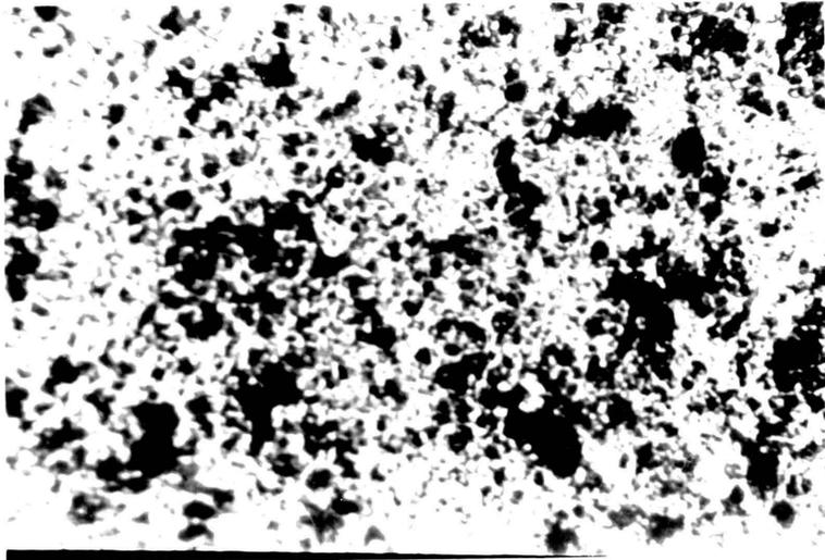
Figure 56- Photomicrograph of a polished section of a specimen from surface showing magnetite with microporous and colloform texture.
